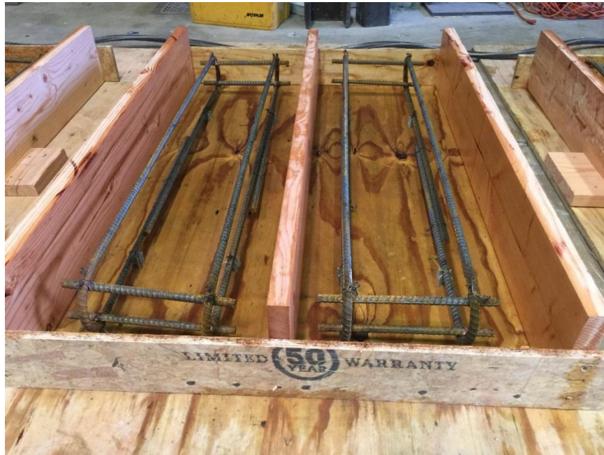
Figure 94. Negative bending flexural test formwork for substrate concrete placement
