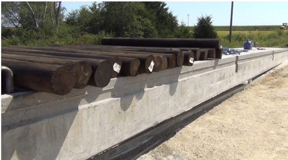
b) The beam when one end was lifted by the tow truck
