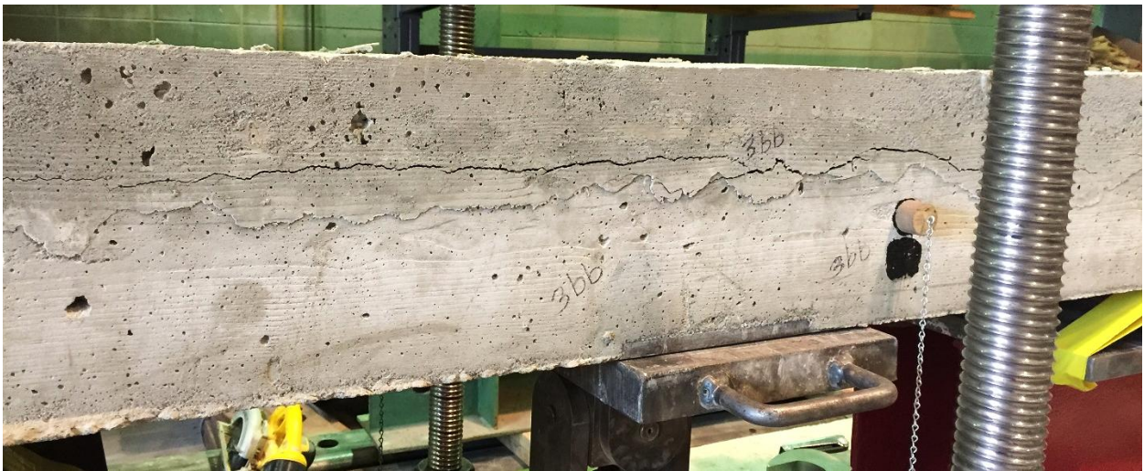
Figure 88. Case 3 positive bending flexural test specimen failure at concrete bond interface
