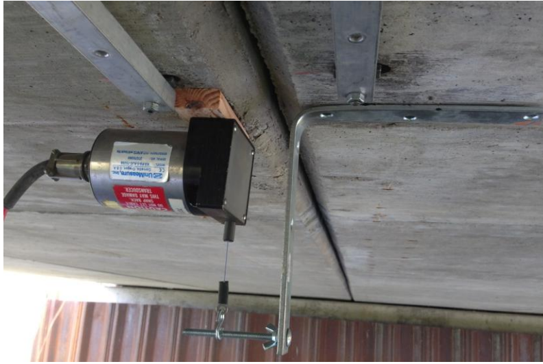
Figure 29. Relative displacement gage setup
