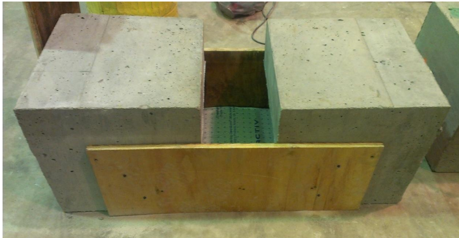
Figure 68. Push-out test formwork for overlay concrete placement
