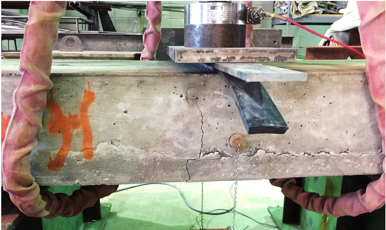
Figure 99. Case 1 negative bending flexural test specimen failure at concrete bond interface
