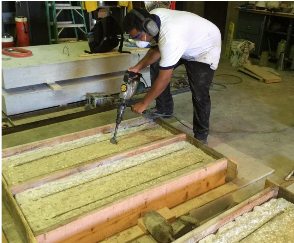
Figure 95. Chipping of substrate concrete for negative bending flexural tests
