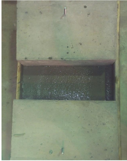
Figure 70. Push-out test specimen after overlay concrete placement
